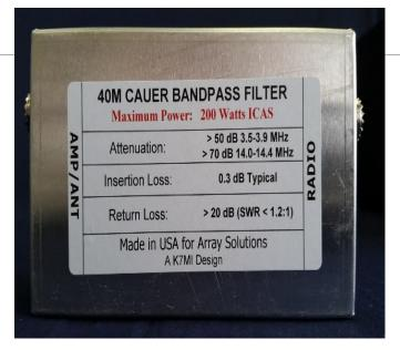
Combined with individual 20m notch stub, total attenuation at 14.300 will be aprox 92db, with insertion loss at aprox .4db
