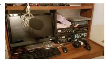
I took Oscar into my shack and showed him the setup, including the MFJ-949E tuner, ANAN-100D software defined radio (shout out to K5JAE!) and all-in-one computer I use to operate. I fired up the radio and PowerHPSDR software and tuned around the 20 meter and 40 meter bands.
